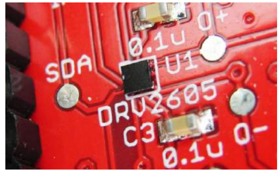
Figure 6. DRV2605 Haptic Driver
