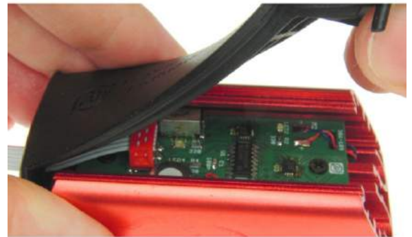
Figure 10. Haptic Grip Peeled Back
