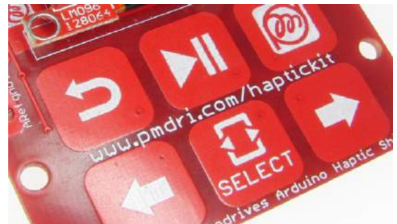
Figure 4. Capacitive Touch Buttons
