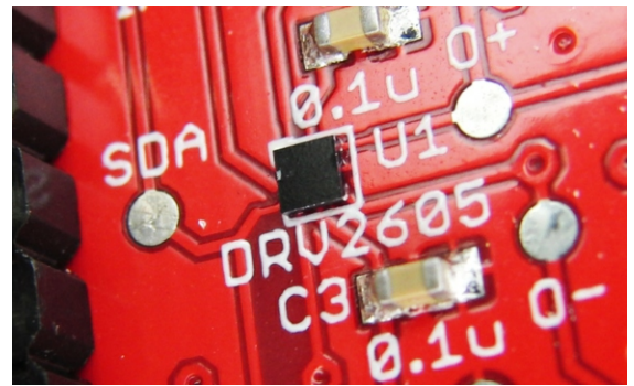
Figure 6. DRV2605 Haptic Driver
